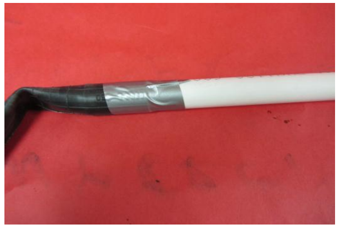
Cut the bike tube. Slide one end onto the end of a PVC pipe and tape in place.
