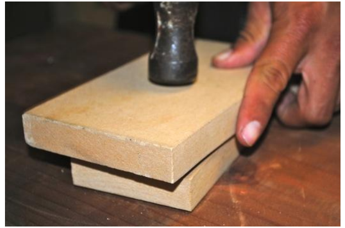
Hammer a 2 nd piece of wood onto the nail.
