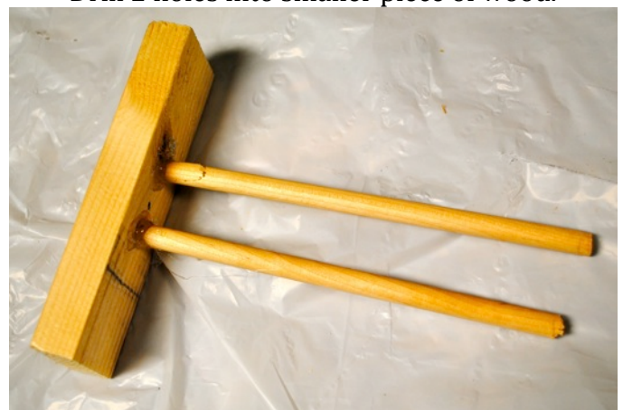
Drill 2 holes into smaller piece of wood.
