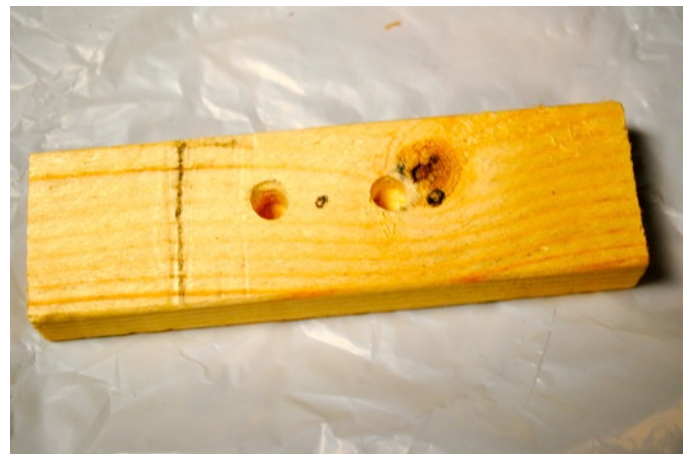
Drill 2 holes into smaller piece of wood.
